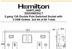
Insert Type 2 gang 13A Double Pole Switched Socket with 2 USB
