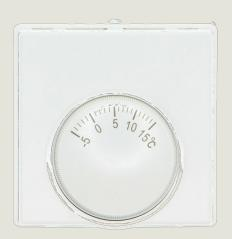
Designed for wall mounting, with 60mm fixing centres for back-box compatibility, and suitable for in-wall or surface- run wiring connection. The thermostat cover incorporates four breakouts for surface-run conduit. The temperature regulation mechanism is the well-proven sealed bellows system. Install in parallel to the room thermostat in a cool area of the property, to protect the property, heating system and boiler against the risk of damage from frost.
